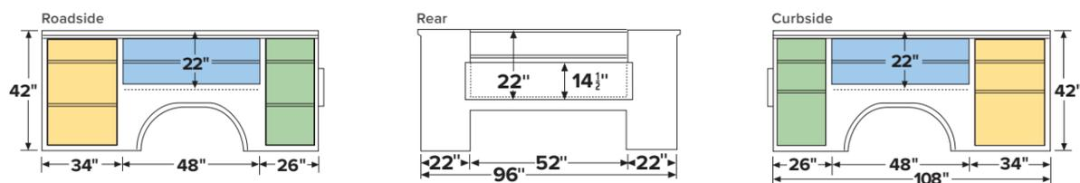
MM225 - Built for a crane rating up to 5,000 lbs. (38,000 ft. lbs.)
