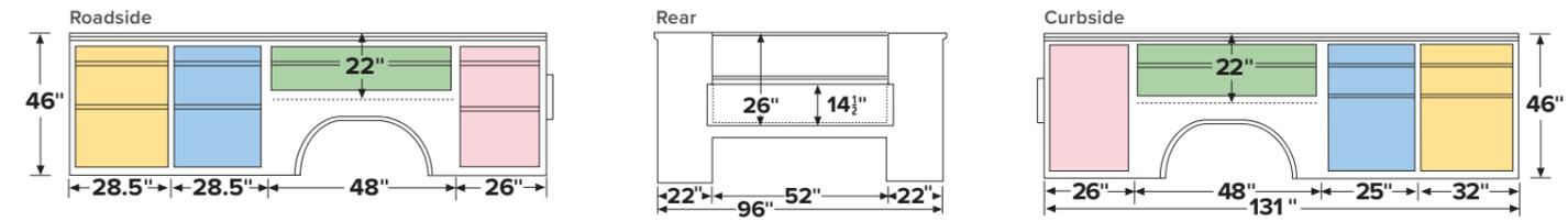
MM278 - Built for a crane rating up to 12,500 lbs. (80,000 ft. lbs.)
