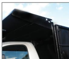
**Fully Welded Cab Guard**
