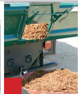
Optional sliding center patchgate controls material flow.
