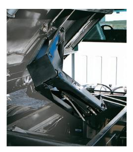
The power behind the Deuce is a double-acting Lo-Boy® hoist on a bayonet swivel. The additional double-acting power allows the Deuce to lift larger loads-up to 11 ton capacity!
