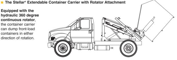
The center of gravity of the ECCR unit is located approximately 9.25" in front of the rear axle. In the stored position, the center of gravity of the container is located approximately 45" behind rear axle.
