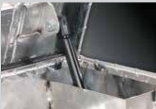
Gas shock cover support protects shocks from damage.
