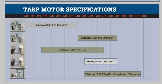
\*All tarp motors can operate on less length then recommended, but they will operate slower than the recommended tarp motor.
