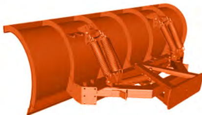
10-Gauge Steel Construction with Extension Springs (STMX1)
