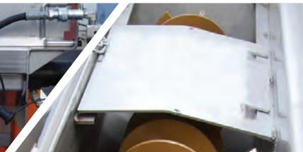
Anti-flow plate prevents material free flow and helps minimize material waste.
