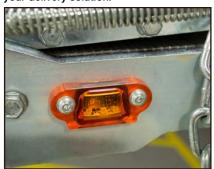
Platform Warning Lights are standard on all WDV GEN II models to provide added safety and security. The lights automatically flash when the liftgate is in operation.
