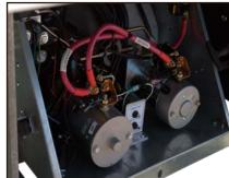
Dual Pump and Motor on 5,500 lb. and 6,600 lb. models with simple toggle to backup. STD Feature.
