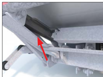
Lift cylinders store in a retracted position behind protective plating, shielding them from road debris that causes pitting.
