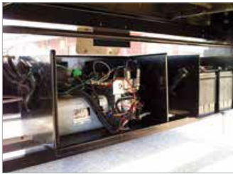
Thermally protected power unit
