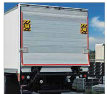
BZ Series Gate in Stowed Position
