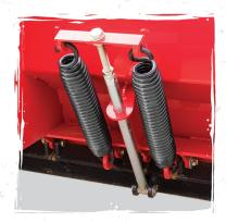
Adjustable, Heavy-Duty Trip Springs are torture-tested and allow the operator to adjust trip-edge tension according to the job at hand.
