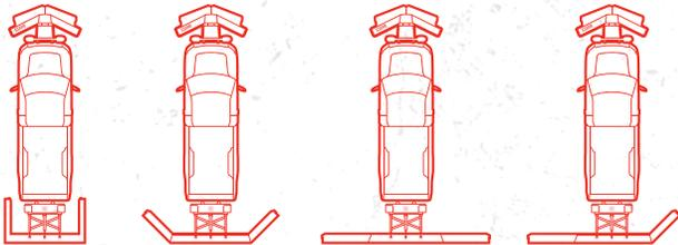
Multiple wing configurations provide added versatility to quickly and easily clear the job site.
