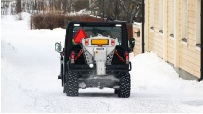
Spreading width up to 30 ft
