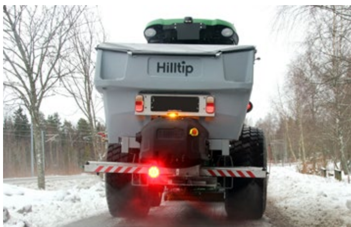
Led work light (red) and beacon light (orange)
