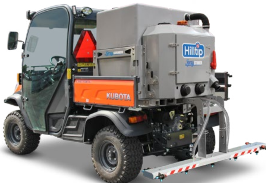
SprayStriker™ 1350 on Kubota utility vehicle
