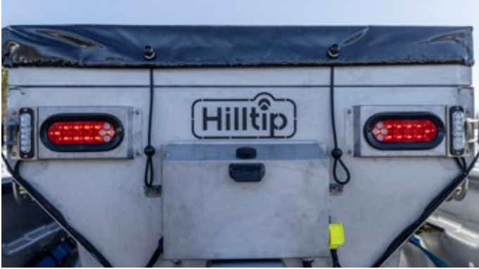
LED Stop/ Tail / Brake lights and strobe lights
