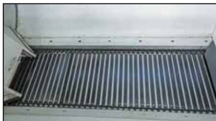
30.25" wide conveyor with 1/2" bars
