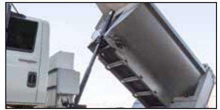
Mailhot® multi-stage, double-acting, nitrified cylinder, trunnion-mounted hoist
