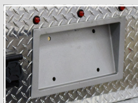
Cast Aluminum License Plate Holder
