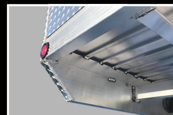
Rear Light - Underside (No Exposed Wiring)
