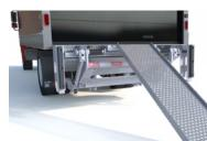
Optional walk ramp can be operated without moving the liftgate.
