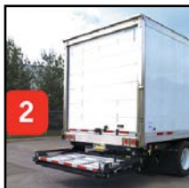
2 Powers Out from Under Trailer
