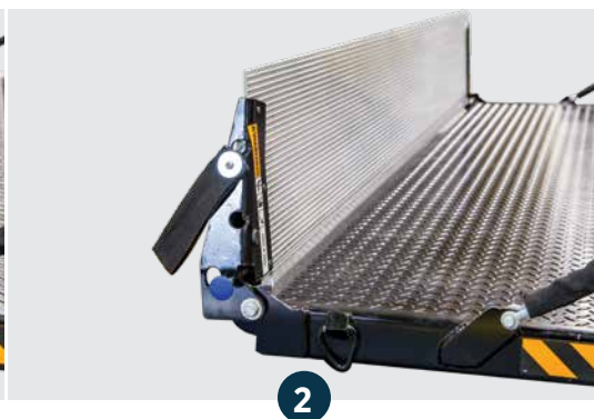
2 ramp locks at 90-degrees for cart retention
