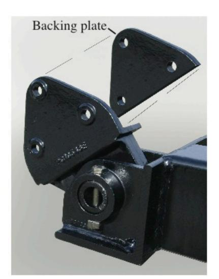
The 834SF's hinges are cast from extra heave duty 4140 grade steel to ensure durability. Adding to the ease of installation and durability, these hinges are bolted then welded to the bodies longitudinals.
