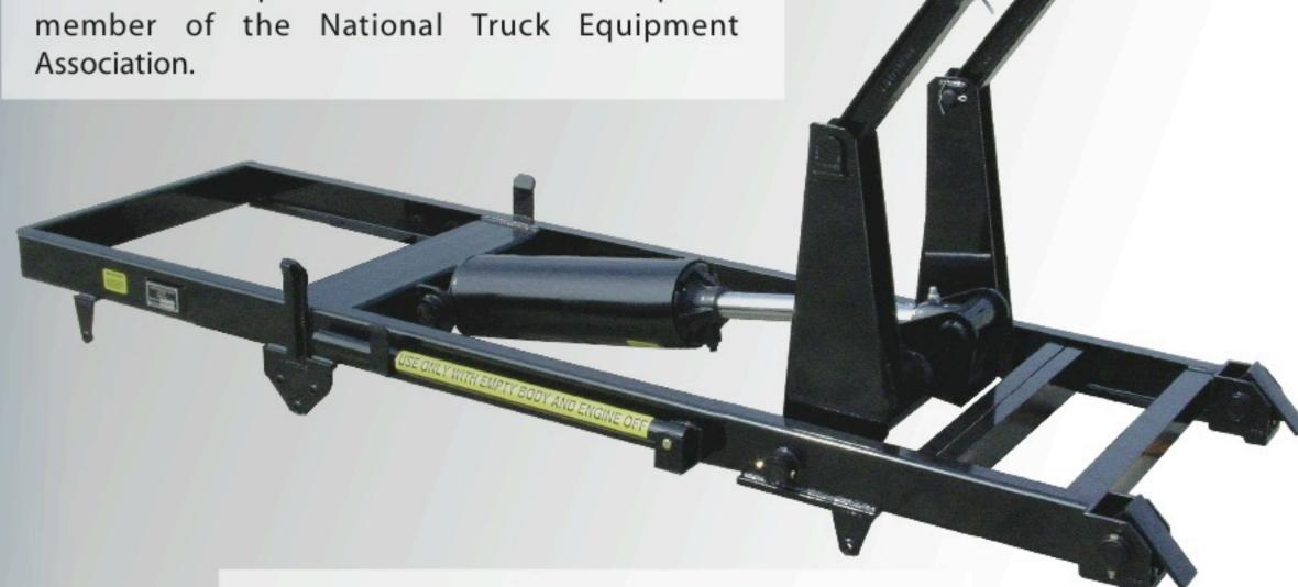
Champion built cylinders and hoists are designed to be double acting (power up and down). Our hoists are easy to install with as little truck and body modification as possible. To further ease the installation process, Champion hoists mount to the body and truck chassis using heavy duty grade 8 bolts with little or no welding needed.
