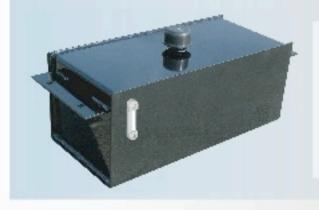
The 8.5 gallon box type reservoir is designed to be frame mounted intank. It hangs out of the way and is equipped with a brass wire mesh suction strainer, oil level & temperature gauge.
