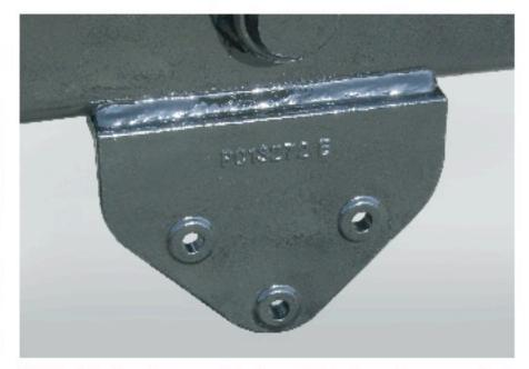
This hoist is easily installed to the trucks chassis using extra heavy duty 4140 grade cast mounting brackets. With 14 grade 8 bolts and minimal welding, installation is quick and easy.
