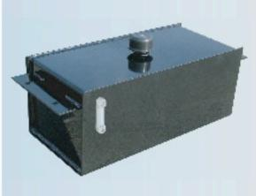
The 8.5 gallon box type reservoir is designed to be frame mounted inboard. It hangs out of the way and is equipped with a brass wire mesh suction strainer, oil level & temperature gauge.
