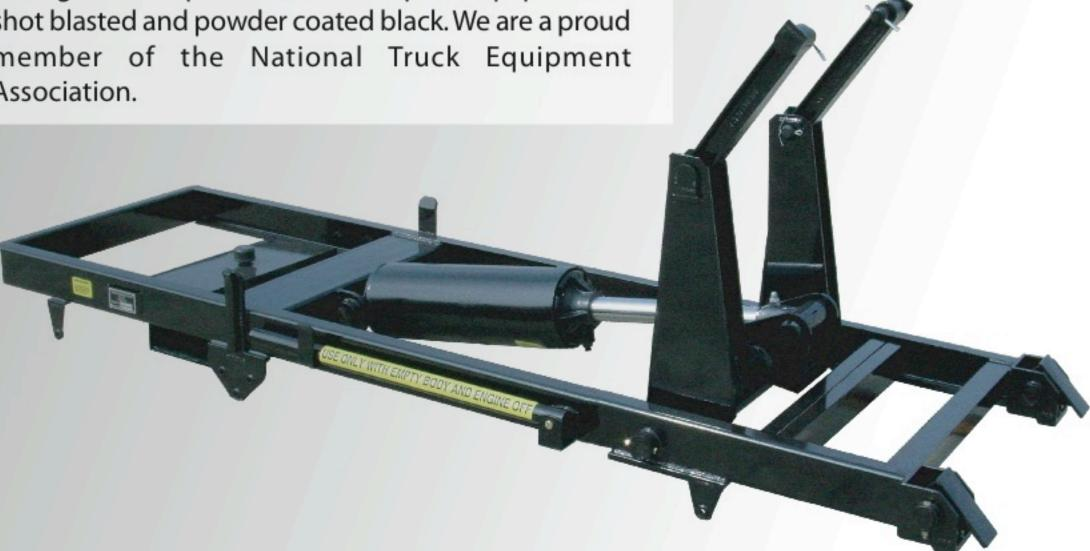
Champion built cylinders and hoists are designed to be double acting (power up and down). Our hoists are easy to install with as little truck and body modification as possible. To further ease the installation process, Champion hoists mount to the body and truck chassis using heavy duty grade 8 bolts with little or no welding needed.
