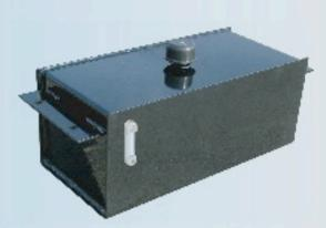
The 8.5 gallon box type reservoir is designed to be frame mounted inboard. It hangs out of the way and is equipped with a brass wire mesh suction strainer, oil level & temperature gauge.
