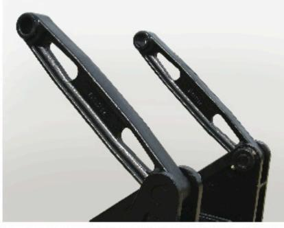
Shown is the 834SF heavy duty cast lift arms. These arms easily attach directly to the body using 4140 grade, 1 1/2" pivot pins which are bolted in place with grade 8 bolts.
