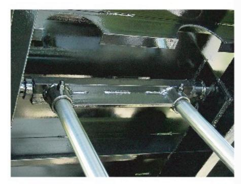
The upper lift point of the 5530DM uses 2 1/4" pins that are welded to the longitudinals for extra strength.
