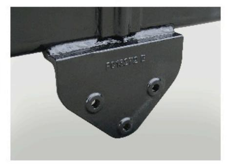
This hoist is easily installed on the trucks chassis using extra heavy duty 4140 grade cast mounting brackets, with 12 grade 8 bolts and minimal welding. Installation is quick and easy.
