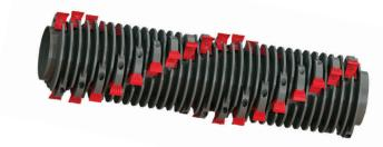
Ideal when you need to process material into a fine end product. The depth control rings provide a smaller bite to create a fast cut with less horsepower draw. The DCR is not recommended for sandy and rocky environments or a job where you may engage the ground; this can cause faster wear.
