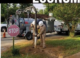
The Mudslinger<sup>™</sup> MS500 and MS800 trailermounted units are designed to provide operators with an economical, portable, and powerful system.
