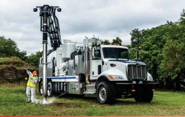
The X-Cavator<sup>™</sup> CXT is the legacy Vac-Con hydrovac. This unit was designed with the power and performance expected from Vac-Con machines with a focus on hydroexcavation applications.
