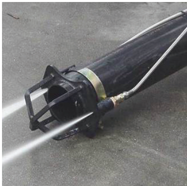
The DSB- 3 " & 4 " combine high pressure water with vacuum to suck a round hole in the ground. Coupled with our Core Drill, it allows digging without using a jackhammer on the pavement.
