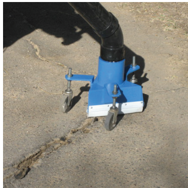
Intended to suck up debris from cracks in the pavement, the crackhead can be used with any sized "Power-Vac"
