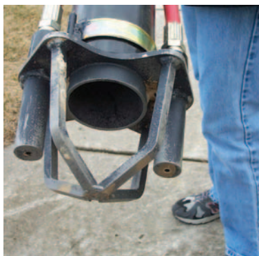
The DSB-AIR-3" & 4" combine high pressure air with vacuum to suck a round hole in the ground.
