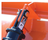
APPROX. ATTACK ANGLE ADJUSTMENT: 5°, 10°, AND 20°
