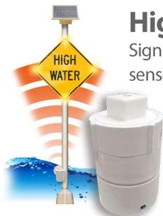
**High Water Sensor** K&K Systems' Sign Alerts can be equipped with a high water sensor for locations known for flooding. When water levels rise above the sensor, the Sign Alerts LEDs are activated. The system is deactivated once the water level lowers below the sensor.
