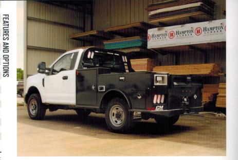
NOTABLE OPTIONS INCLUDE: 3/16" Heavy-Duty Deck; 30K B&W Hitch with Turnover Ball (required for 5th Wheel capability); Bale Spikes; Color Primer Only; Stainless Fenders; Work Lights (standard on TM Deluxe)
