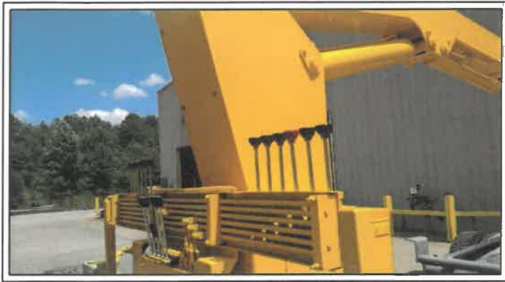
Bolt-On Bucket Cylinder Covers & Reversible Bolt-On Bucket Edges
