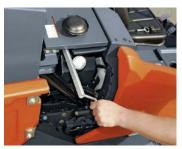
Wear compensation made easy: The main sweeping cylinder can be adjusted by means of the Automatic-Hopper-Broom-Adjustment system for a perfect sweeping pattern throughout the entire life cycle of the cylinder.
