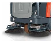
Robust chassis and collision protection: The chassis provides a solid base and collision-protected brooms ensure highest possible machine reliability.
