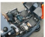
Easy maintenance: To carryout maintenance work, the forward-opening operating panel provides easy access.
