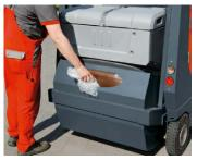
Practical coarse dirt flap to throw-in larger piecesof debris, plastic films or straps. No dust can escape when opening the coarse dirt flap.
