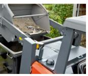
Hydraulic High-Dump Option: The dirt hopper allows high dumping at heights of up to 60".
