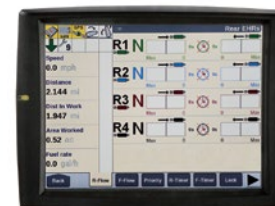
Overview of flowrate and timer settings on the AFS Pro 700 display.
