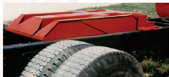
Hoist mounts low between the frame, meaning no notching crossmembers under dump body.
