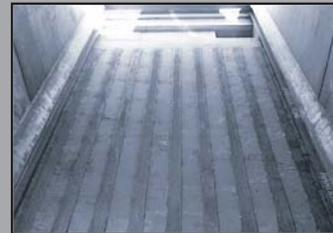
*The blade travels just above the body floor on cam followers to reduce floor wear. T1 strips hold commodity up, which prevents it from going under the blade and also reduces floor wear.*
