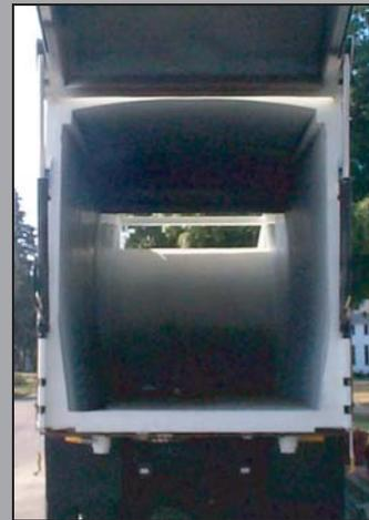
*The contoured blade follows the continuous uniform side walls from compactor through the body smoothly and completely clean.*
