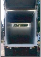
The contoured blade follows the continuous uniform side walls from compactor through the body smoothly and completely clean.
