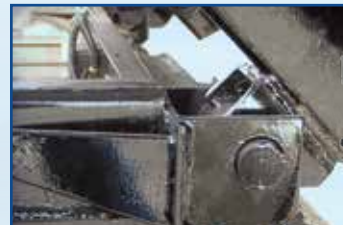
The Yardbird's heavy-duty platform hinge is greasable.
