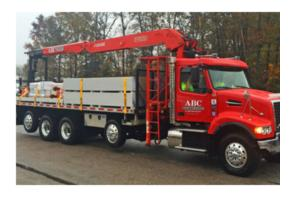
booms in higher-performance models. The models in this range cannot assume the classic rest position with the crane completely closed behind the truck cabin due to the length of the main arm. Consequently, their rest position is with the main and secondary arms aligned along the truck bed and the hook on a support at the rear of the truck.
