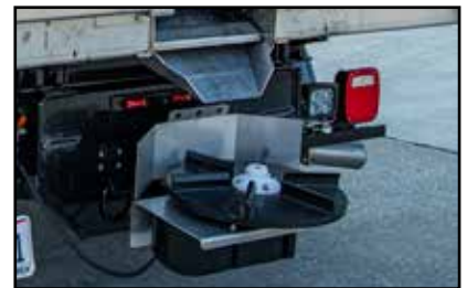
Removable spinner assembly for easy switch between spreader and dump applications
