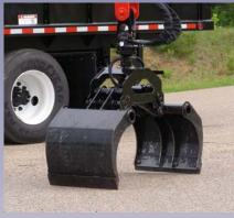
The boom is equipped with a continuous rotating grapple. The grapple is constructed with bolt-on heat-treated steel cutting edges for ease of replacement. The edges are overlapping to prevent scalping. The bucket is 36" wide with a 48" opening from lip to lip.
