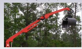
The boom is a 17 foot fixed boom constructed with a one piece main boom.
