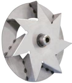
Powerful 7- or 9- blade fan and steel impeller produces high airflow while the scrolled housing allows uninterrupted air intake. Even if a portion of the housing is covered with leaves and debris, airflow can still enter the impeller area and be forced out the discharge chute.
