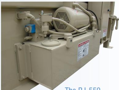
The RJ-550 features Marathon's side-mounted power unit. The power unit offers the convenience and ease-of-maintenance of a remote power pack with the space savings of an integrated power pack. The configuration also eliminates ALL electrical components from inside the compactor.
