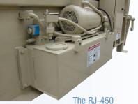
features Marathon's side-mounted power unit. The power unit offers the convenience and ease-of-maintenance of a remote power pack with the space savings of an integrated power pack. The configuration also eliminates ALL electrical components from inside the compactor.
