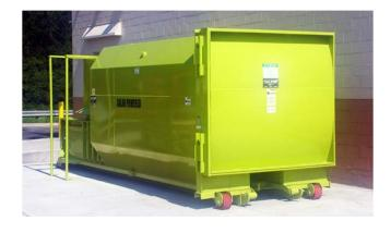
This bottling plant in Virginia has a Green Built Hybrid solar-powered RJ-250SC self-contained compactor with a side-feed security chute.
