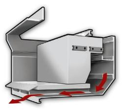
The Qwik Clean® Tank feature, standard on all RJ-250SC compactors, funnels any liquid seepage which can occur during compaction into an enclosed area underneath the charge box floor. The liquid is automatically discharged at the disposal site, in effect flushing the container and the area behind the ram. The 12-inches (305mm) high, up to 750-gallon (2839) liters) capacity sump area is designed to provide easier hook access for roll-off drivers.
