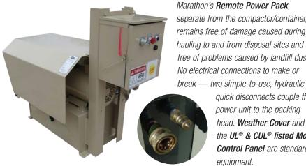
Marathon's Remote Power Pack. separate from the compactor/container, remains free of damage caused during hauling to and from disposal sites and free of problems caused by landfill dust. No electrical connections to make or
