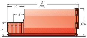
Dimensions not shown: 8' 4½" (2543mm) Overall Width Ground Roller Widths: 61½" (1569mm) Inside Rollers 67½" (1712mm) Roller Centers 72½" (1851mm) Outside Rollers
