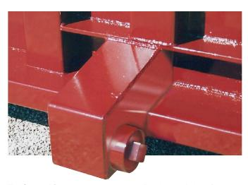
The **StreamLine** option enables excess liquid to be drained from the container, reducing net payload weight and significantly reducing hauling costs. Liquid is routed to four interconnected 4" (101.6mm) drain outlets located at each corner of the StreamLine unit. Connection can be made to a hose, piping, or a pump.
