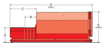
Dimensions not shown: 8' 41/8" (2543mm) Overall Width Ground Roller Widths: 61 1/8" (1569mm) Inside Rollers 67 1/8" (1712mm) Roller Centers 72 1/8" (1851mm) Outside Rollers
