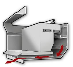
The Qwik Clean® Tank feature, standard on all RJ-100SC compactors, funnels any liquid seepage which can occur during compaction into an enclosed area underneath the charge box floor. The liquid is automatically discharged at the disposal site, in effect flushing the container and the area behind the ram. The 12-inches (305mm) high, 750-gallon (2839 liters) capacity sump area is designed to provide easier hook access for roll-off drivers.
