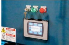
The touchscreen allows full automatic and manual control with one touch. Screens may be customized, password protected, and are designed with alarm, diagnostic and help screens.
