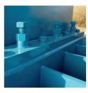
The Galaxy2R® features an adjustable shear beam that enables you to adjust the shear blades from the exterior of the machine.
