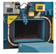
Multi-purpose door can serve as a bale separator, bale release, or bale clamp. It also allows for variable bale widths.
