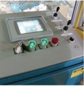
Maestro<sup>™</sup> color touchscreen operator interface PLC programmable controller features automatic and manual controls, diagnostics and bale set-up functions. Available with multilanguage function.
