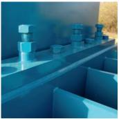
The Galaxy2R® features an adjustable shear beam that enables you to adjust the shear blades from the exterior of the machine.
