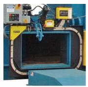
Multi-purpose door can serve as a bale separator, bale release, or bale clamp. It also allows for variable bale widths.
