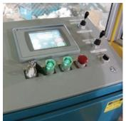
Maestro<sup>™</sup> color touchscreen operator interface PLC programmable controller features automatic and manual controls, diagnostics and bale set-up functions. Available with multilanguage function.
