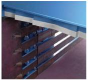
Serrated body and ram bolt-in shear blades are shimmable and replaceable (not available in the PC-Series, WC, and EWC models).
